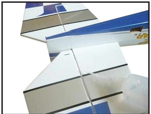
7) Break in the hinges by working the stabilizer up and down a number of times. This will reduce the initial load on the servo when the servo is connected for the first time.
