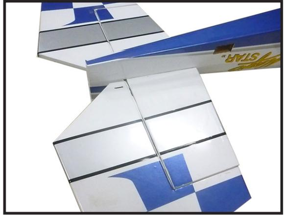
5) Remove the T-pins from hinges. Position the elevators so they move freely without the counterbalances hitting the ends of the stabilizer.
