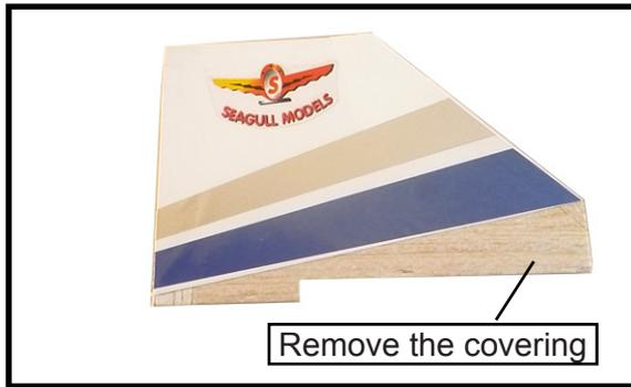
**!** *When cutting through the covering to remove it, cut with only enough pressure to only cut through the covering itself. Cutting into the balsa structure may weaken it.*
