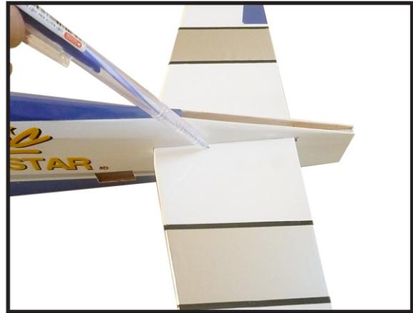
5) Remove the stabilizer. Using the lines you just drew as a guide, carefully remove the covering from between them using a modeling knife.
