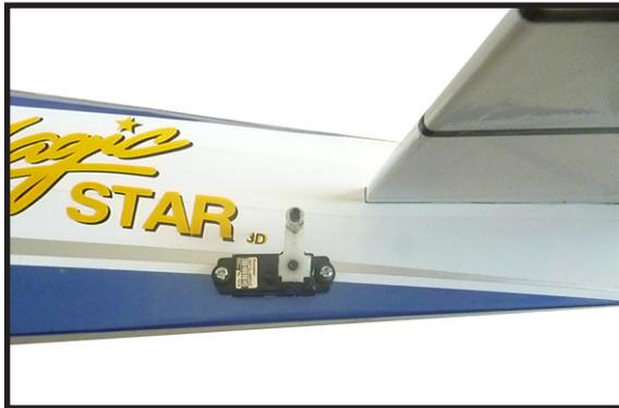
2) Locate position elevator control horn. Then, apply 2-3 drops of epoxy to the backplate where it contacts control horn to keep it from accidentally coming loose in flight.
