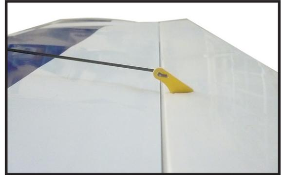
3) The pushrod wire will pass through the hole in the micro screw-lock connector. Use side cutters to trim the pushrod so it is past the connector as shown.
