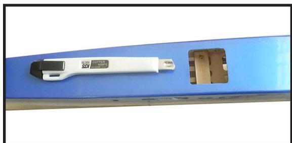
2) Slide the aluminum tube into the socket in the fuselage.
