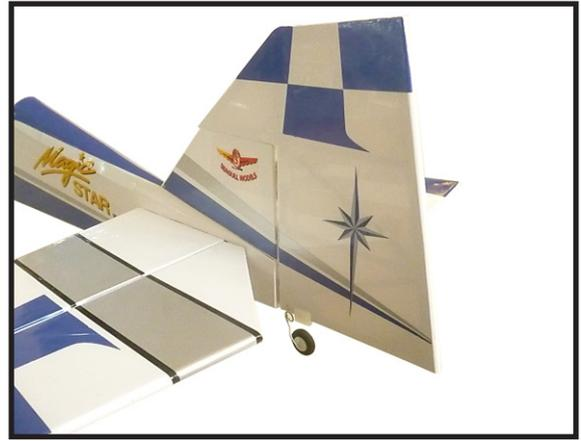
10) Check to make sure the counterbalance can move freely without hitting the top of the fin. Apply thin CA to each of the hinges. Make sure to fully saturate both sides of the hinges.
