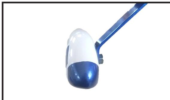
*Repeat steps to install remaining wheel pants to the landing gear.*
