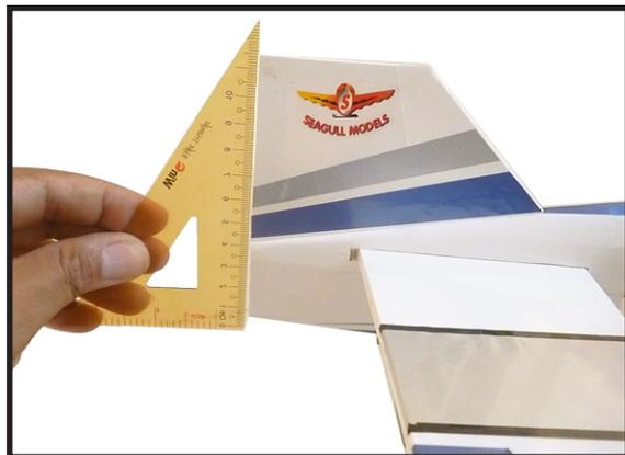
4) When you are sure that everything is aligned correctly, mix up a generous amount of 30 Minute Epoxy. Apply a thin layer to the mounting slot in the top of the fuselage and to the sides and bottom of the vertical stabilizer mounting area. Apply epoxy to the bottom and top edges of the filler block and to the lower hinge also. Set the stabilizer in place and realign. Double check all of your measurements once more before the epoxy cures.
