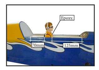
4) Position the canopy onto the fuselage. Trace around the canopy and onto the fuselage using a felt-tipped pen.
