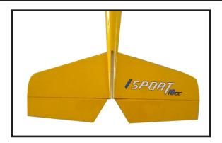
4) With the stabilizer held firmly in place, use a pen and draw lines onto the stabilizer where it and the fuselage sides meet. Do this on both the right and left sides and top and bottom of the stabilizer.
