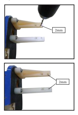
4) On the fire wall has the location for the throttle pusshrod tube (pre-drill).
