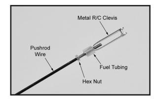
Use a felt tip pen to mark the wire where it crosses the hole. Use a pair of pliers to put a shrp 90-degree bend in the wire at the mark.
