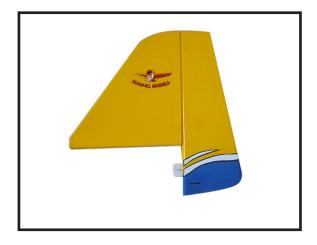
1) While holding the vertical stabilizer firmly in place, use a pen and draw a line on each side of the vertical stabilizer where it meets the top of the fuselage.
