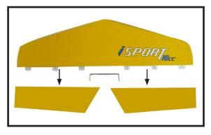
2) Carefully remove the elevator from one of the horizontal stabilizer panels. Note the position of the hinges.
