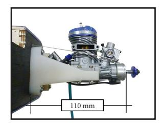
2) Use a pin drill and 2mm drill bit to drill a small indentation in the mount for the engine mounting screw.
