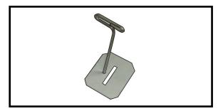
2) Remove each hinge from the wing panel and aileron and place a T-pin in the center of each hinge. Slide each hinge into the aileron until the T-pin is snug against the aileron. This will help ensure an equal amount of hinge is on either side of the hinge line when the aileron is mounted to the wing panel.
