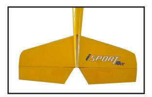
8) After the epoxy has fully cured, remove the masking tape or T-pins used to hold the stabilizer in place. Carefully inspect the glue joints. Use more epoxy to fill in any gaps that may exist that were not filled previously and clean up the excess using a paper towel and rubbing alcohol.
