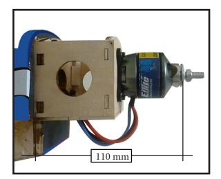
5) Attach the speed control to the side of the motor box using two-sided tape and tie wraps. Connect the appropriate leads from the speed control to the motor. Make sure the leads will not interfere with the operation of the motor.
