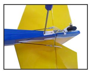
2) Adjust the wheel collar shown to set the height of the tailwheel wire. Then check to see if the long steering leg of the tailwheel wire is parallel to the bottom of the rudder. The wire may need to be tweaked slightly to make it parallel.
