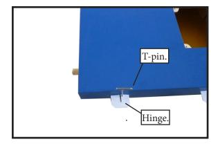
3) Slide the aileron on the wing panel until there is only a slight gap. The hinge is now centered on the wing panel and aileron. Remove the T-pins and snug the aileron against the wing panel. A gap of 1/64" or less should be maintained between the wing panel and aileron.
