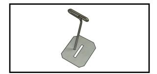
2) Remove each hinge from the wing panel and aileron and place a T-pin in the center of each hinge. Slide each hinge into the aileron until the T-pin is snug against the aileron. This will help ensure an equal amount of hinge is on either side of the hinge line when the aileron is mounted to the wing panel.
