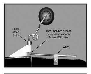
ELEVATOR - RUDDER PUSHROD HORN INSTALLATION.
