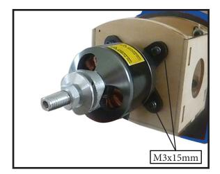
4) Locate the plywood battery tray to the fuselage. Tighten the screws using machine screws M3x15mm to secure the tray in position.
