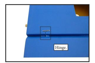
4) Deflect the aileron and completely saturate each hinge with thin C/A glue. The ailerons front surface should lightly contact the wing during this procedure. Ideally, when the hinges are glued in place, a 1/64" gap or less will be maintained throughout the lengh of the aileron to the wing panel hinge line.
