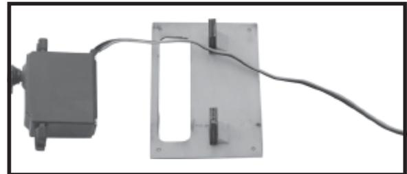
□ 4. Using the thread as a guide and using masking tape, tape the servo lead to the end of the thread: carefully pull the thread out. When you have pulled the servo lead out, remove the masking tape and the servo lead from the thread.
