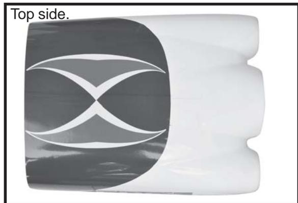
□ 2) While keeping the back edge of the cowl flush with the marks, align the front of the cowl with the crankshaft of the engine. The front of the cowl should be positioned so the crankshaft is in **nearly** the middle of the cowl opening. Hold the cowl firmly in place using pieces of masking tape.
