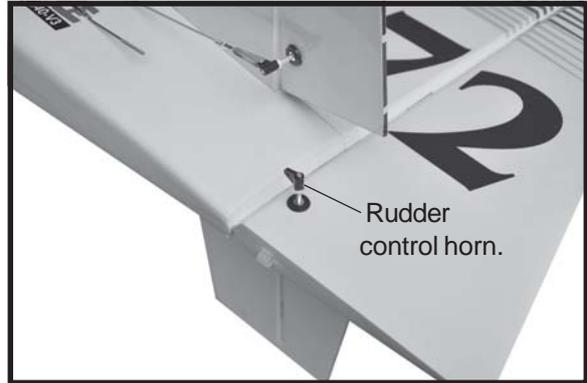
**RUDDER PUSHROD INSTALLATION.**
