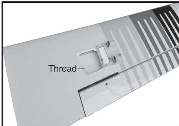
□ 2. Using a modeling knife, remove the covering servo tray.
