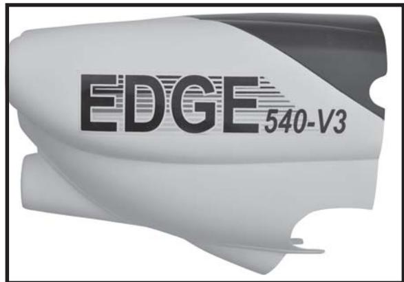
□ 2) While keeping the back edge of the cowl flush with the marks, align the front of the cowl with the crankshaft of the motor. The front of the cowl should be positioned so the crankshaft is in **nearly** the middle of the cowl opening. Hold the cowl firmly in place using pieces of masking tape.
