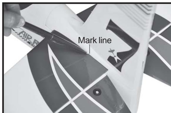
□ 3. Now, remove the rudder and using a modeling knife, carefully cut just inside the marked lines and remove the film of the rudder. Just as you did with the horizontal stabilizer, make sure you only press hard enough to cut the film, not the balsa rudder.
