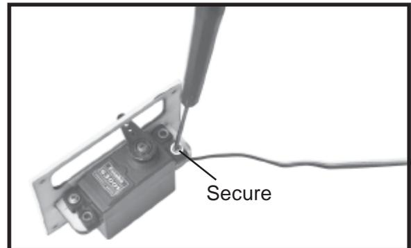
□ 5. Instal servo tray with aileron servo into the wing as same as picture below.
