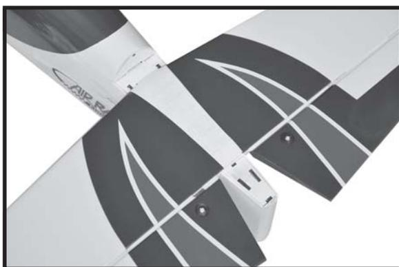
□ 4. Put the vertical stabilizer back in place. Using a triangle, check to ensure that the vertical stabilizer is aligned 90 degree to the horizontal stabilizer.
