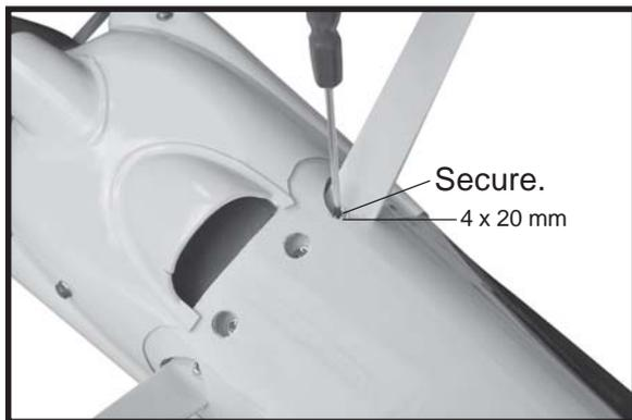
□ 2) Using the hardware provided, mount the main landing gear to the fuselage.
