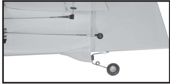
Plastic parts of rudder and elevator pushrod.
