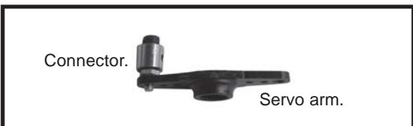
*After installing the adjustable metal connector apply a small drop of thin C/A to the bottom nut. This will prevent the connector from loosening during flight.*
