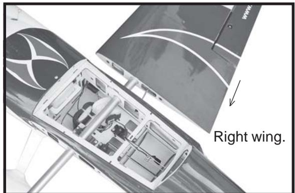
See picture wing attach to fuselage.
