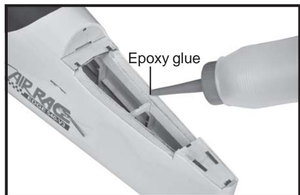
□ 5. When you are sure that everything is aligned correctly, mix up a generous amount of 30 minute epoxy. Apply a thin layer to the top and bottom of the stabilizer mounting area and to the stabilizer mounting platform sides in the fuselage. Slide the stabilizer in place and re-align. Double check all of your measurements one more time before the
